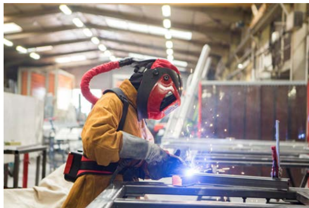
An example of personal fume extraction
